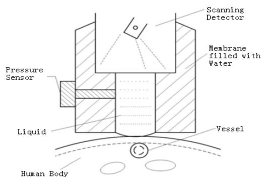
**Figure 1:** Non-pressure Arm Bath-tube
