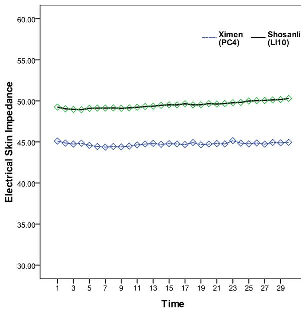
Figure 4: Repeatability of device during a 30 minute period
